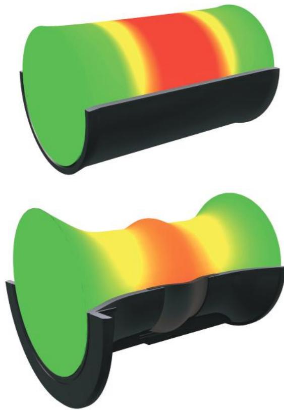
Figure 8 Pressure of the first "organ pipe" resonance in a port Top – rigid walls and no end flare Bottom – flexible walls and end flares
